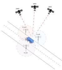
complementary trade-off between them, since on GNSS positioning we have a better accuracy while on 5G positioning we have a better latency, so joining them together we can have the better of both technologies.
