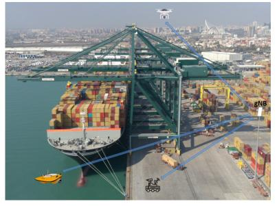
The UAV, USV, and UGV will coordinate to monitor port access areas, anchoring zones, and critical infrastructures to ensure port security. A specific scenario will simulate a coordinated threat response involving an unauthorized boat entering the port and discharging people and goods onto the shore. Both maritime and aerial assets will act in concert to respond to this threat by conducting simultaneous surveillance, identification, and interception tasks.
